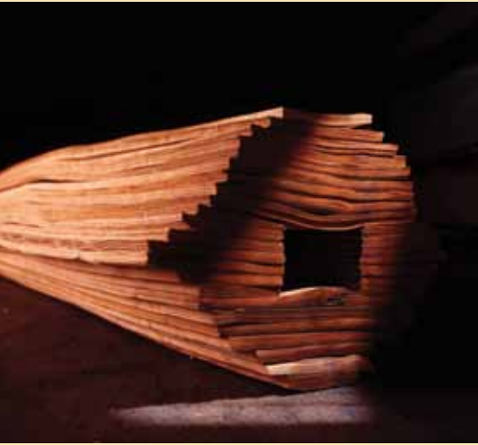
Veneer sliced and assembled in the shape of the log from which it came.
